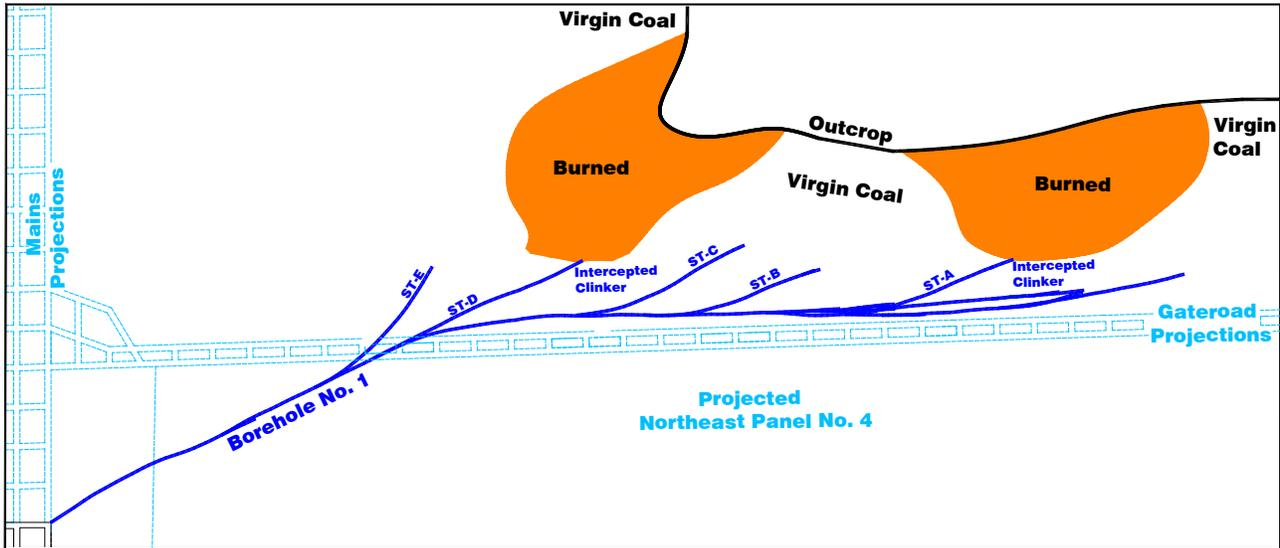
**Figure No. 5:** Plan view illustrating the directional drilling effort performed to characterize the extent of burn into the reserve. Note the exploration side-tracks developed from the main borehole to define the distance between competent coal, as verified by the main borehole, to the burn.
