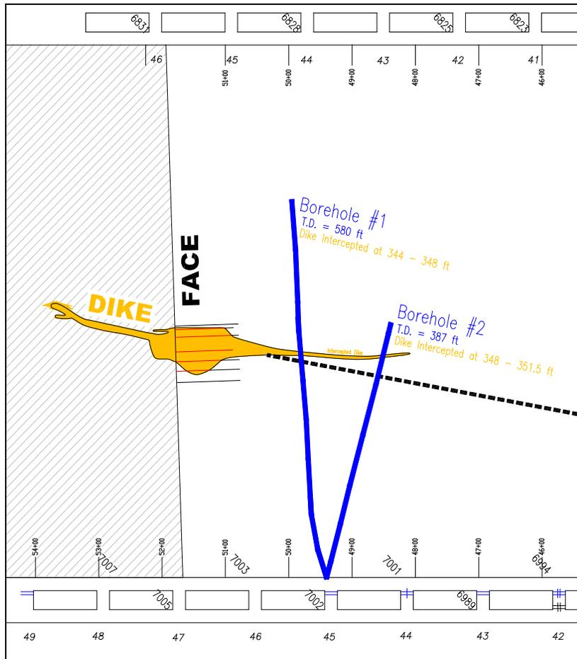
**Figure No. 6:** Plan view illustrating the directional drilling effort performed to characterize the extent of the igneous intrusion in by the longwall face. Note that face drilling indicated the dike was massive and extended in by.
