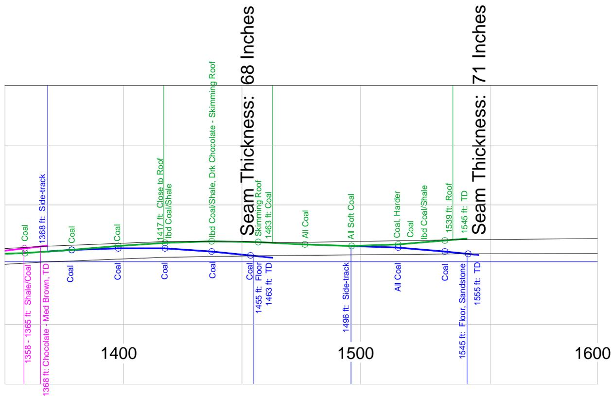
**Figure No. 2:** Profile view of the initial borehole (green) and side-tracking (blue) to determine seam height using horizontal directional drilling (HDD). Note the proximity of the floor touches relative to the roof touches and the level of detail ascertained from drilling logs and borehole survey data.
