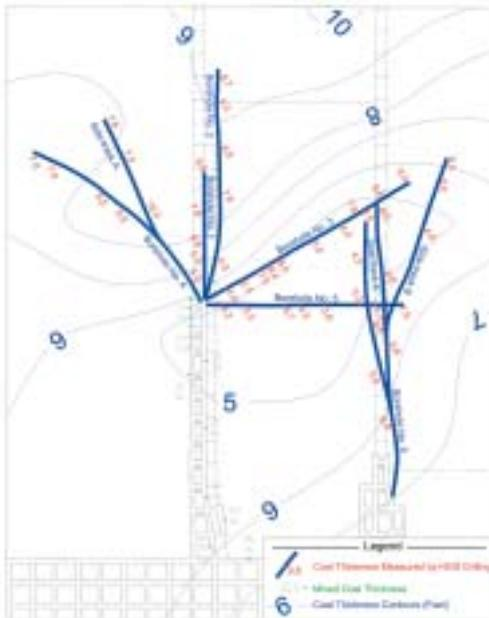
This technique relies on coinciding roof and floor contact points, the use of proper borehole surveying techniques, and interpretation of the roof and floor through drilling thrust, downhole water pressures and cuttings. Using these parameters, REI has provided mine operators with reasonable predictions of the seam profile and the extent of post-depositional features which have been validated by subsequent mining.
