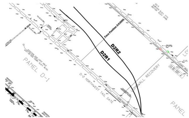
Figure 2. HGBs drilled over the D2 longwall panel at the Willow Creek Mine, Utah, USA.
