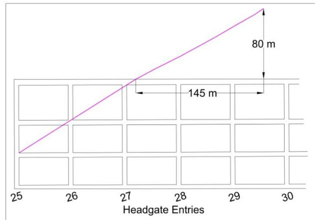
Figure 6b: Plan view of the best performing headgate modified cross-measure borehole at WLM1.
