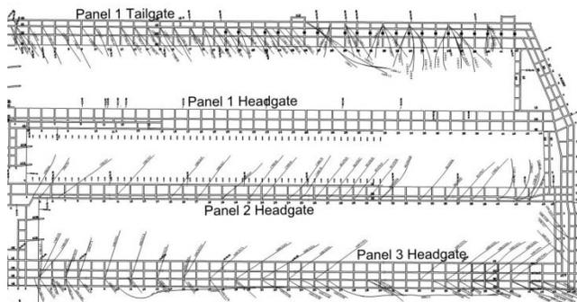
Figure 4. Conventional cross-measure and modified cross-measure HGBs at WLM1.
