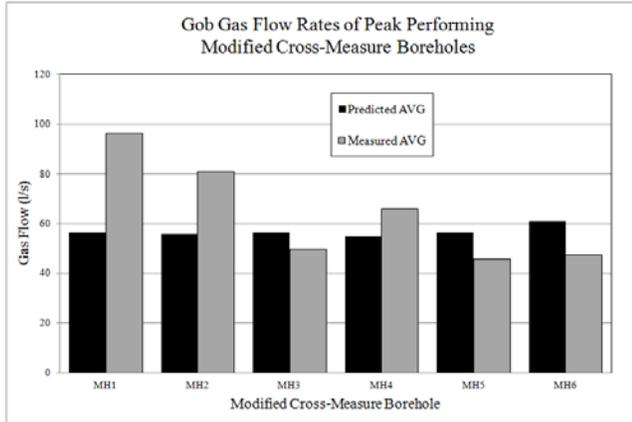
Figure 7. Measured vs. predicted average gob gas flow for best performing modified cross-measure boreholes.
