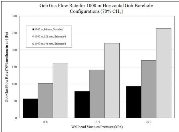
Figure 8. Gob gas flow rate projections for high capacity HGB configurations at varying wellhead vacuum.
