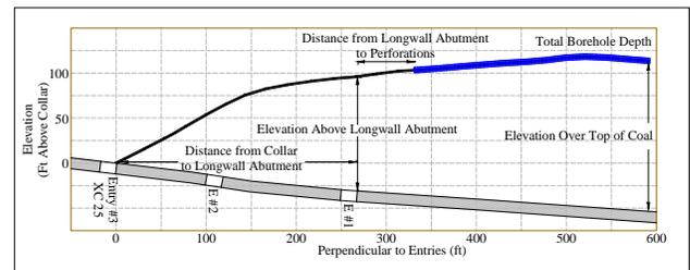
Figure 5a: Parameters that affect modified cross-measure borehole performance.
