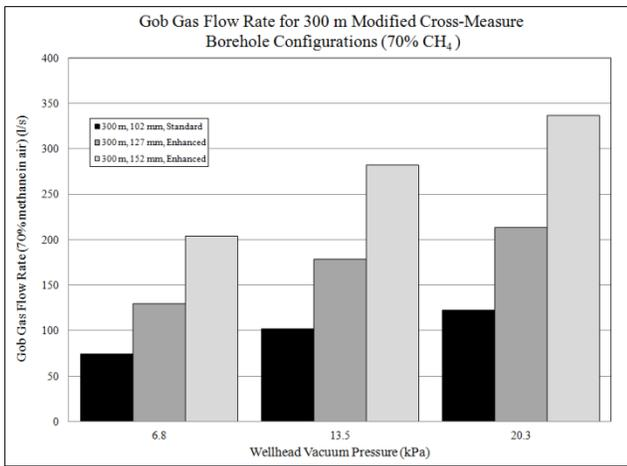
Figure 8. Gob gas flow rate for high capacity modified cross-measure borehole configurations at varying wellhead vacuum.
