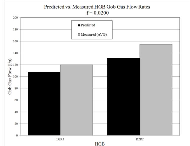
Figure 3. Measured vs. predicted gas flow for boreholes D2R1 and DR2.
