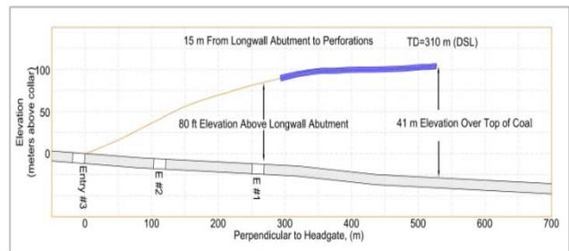
Figure 6a: Cross-section of the best performing headgate modified cross-measure boreholes at WLM1.
