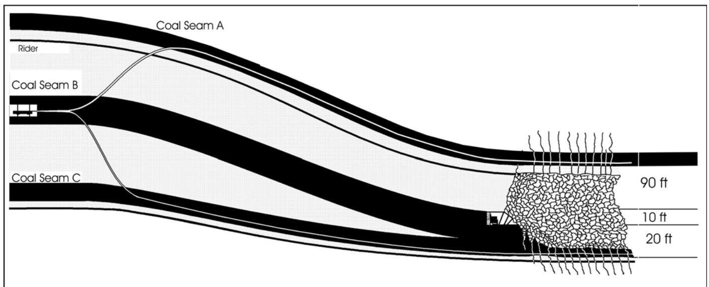
Figure 2. Dual purpose overlying borehole reduces gas contents of gob gas contributing source seam in advance of undermining and subsequently serve as gob boreholes.
